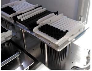
Removable rack with different sized tips and sheaths for the magnetic head.
