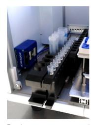
Ready to use reagents and up to 48 samples charging, integrated barcode reading for sample traceability.
