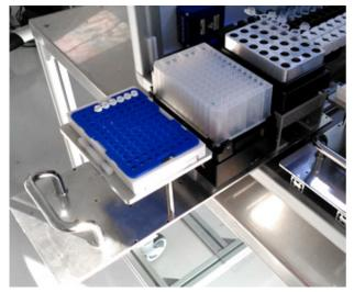
Removable rack with temperature controlled zone for dedicated reagents (heating and cooling unit), thermoshaker (for sample lysis and elution) and PCR set-up plate.
