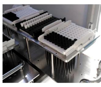
Removable rack with different sized tips and sheaths for the magnetic head.
