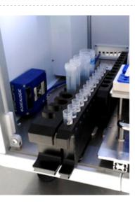
Ready to use reagents and up to 48 samples charging, integrated barcode reading for sample traceability.
